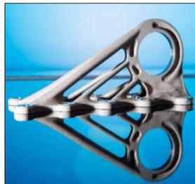
*Additively manufactured developmental bracket produced by Airbus for the A350 XWB aircraft*
